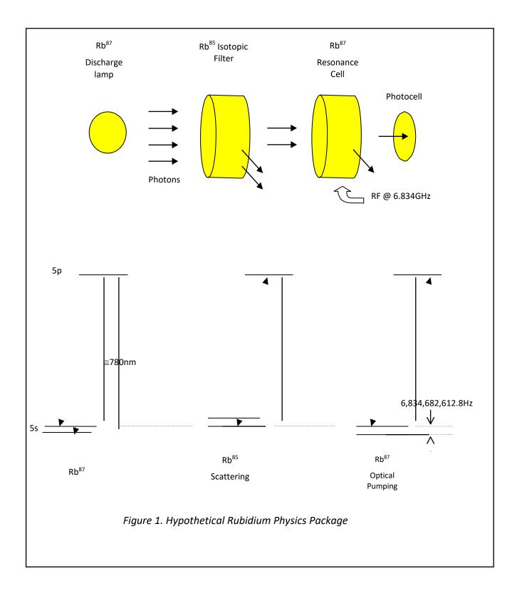
Now, if we apply a microwave field at the frequency corresponding to the hyperfine transition frequency (6.834,682,612,8 GHz), the populations in the ground state will mix, and the amount of light reaching the photodetector will decrease.
